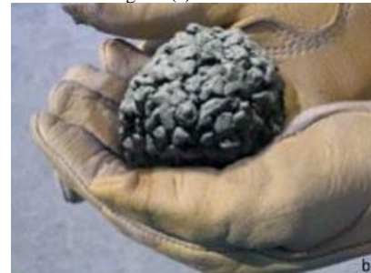
Fig 3.3 (b). Correct amount of water
