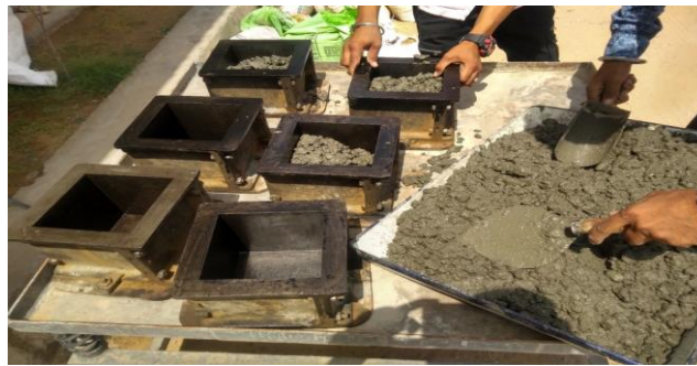
Figure 2.2 Casting of Specimens
