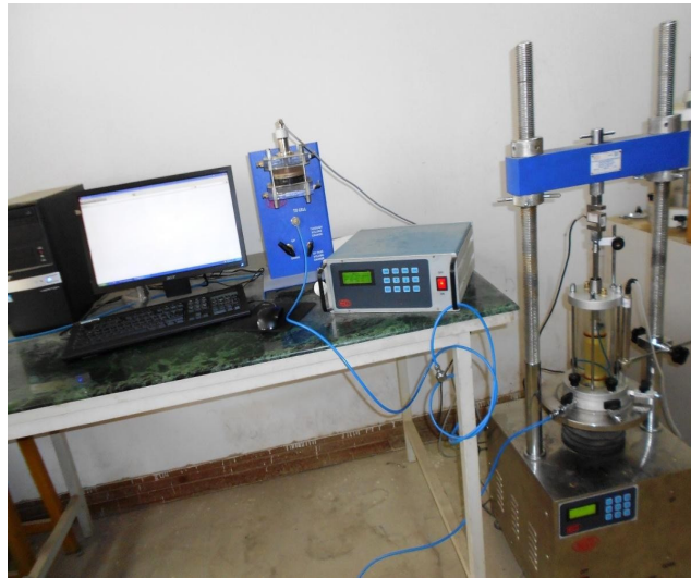
Fig. 2.2.5 Photographic view of the triaxial test set up
